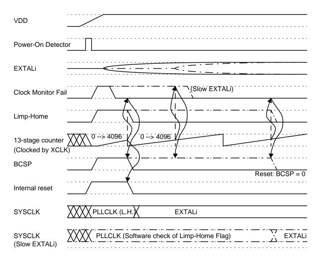
Figure 16 No Clock at Power-On Reset
