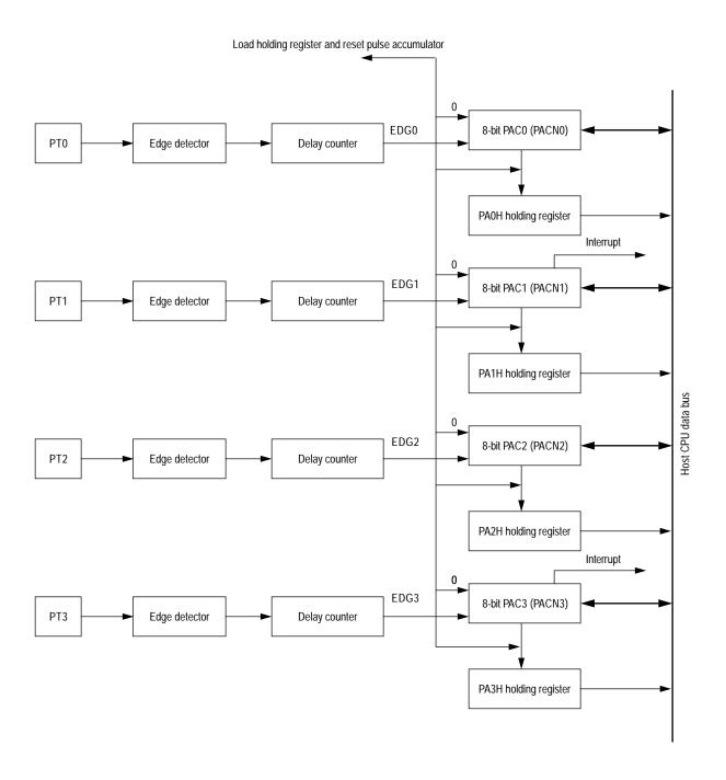
Figure 28 8-Bit Pulse Accumulators Block Diagram
