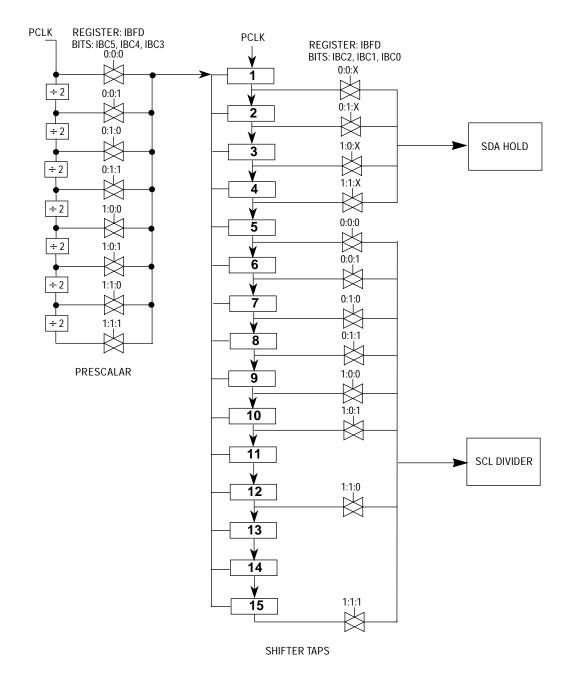
Figure 20 Clock Chain for IIC
