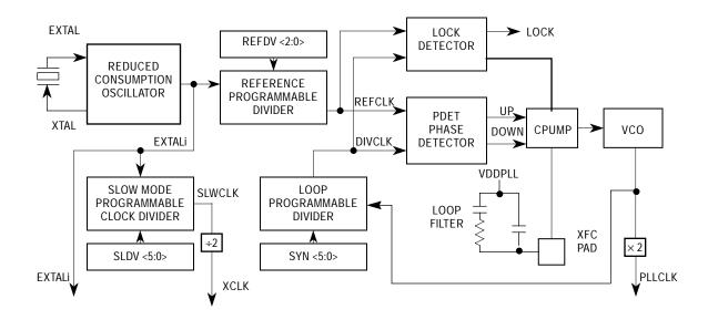
Figure 14 PLL Functional Diagram
