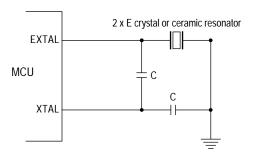
Figure 5 Common Crystal Connections
