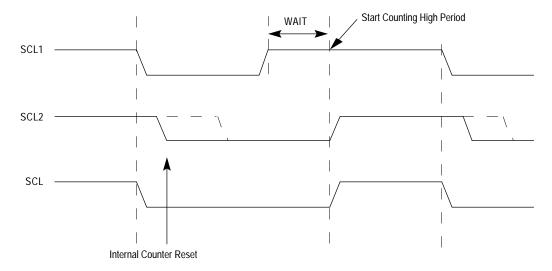
Figure 40 IIC Clock Synchronization
