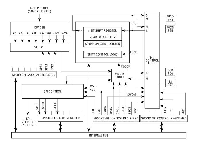
Figure 34 Serial Peripheral Interface Block Diagram
