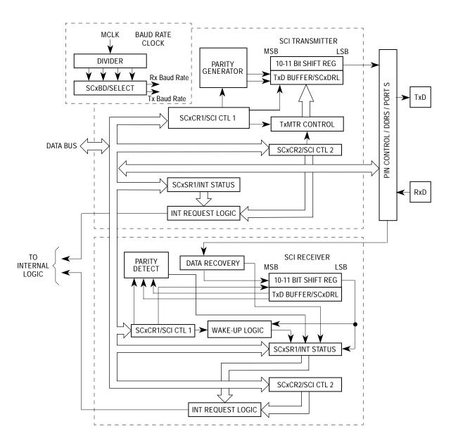
Figure 33 Serial Communications Interface Block Diagram
