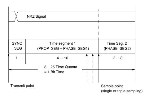
Figure 50 Segments within the Bit Time
