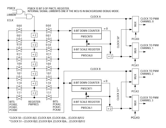
Figure 25 PWM Clock Sources
