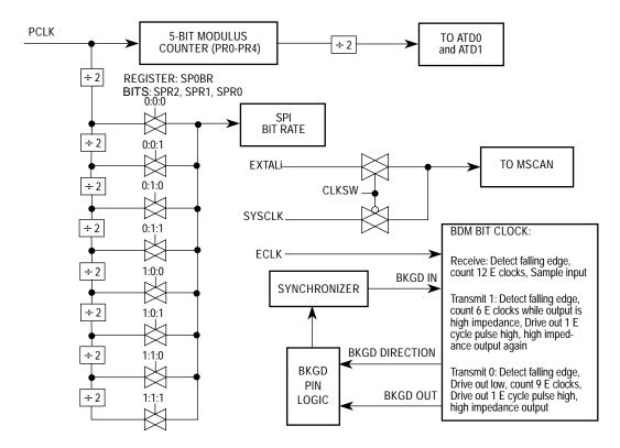
Figure 22 Clock Chain for MSCAN, SPI, ATD0, ATD1 and BDM
