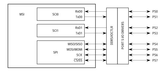
Figure 32 Multiple Serial Interface Block Diagram
