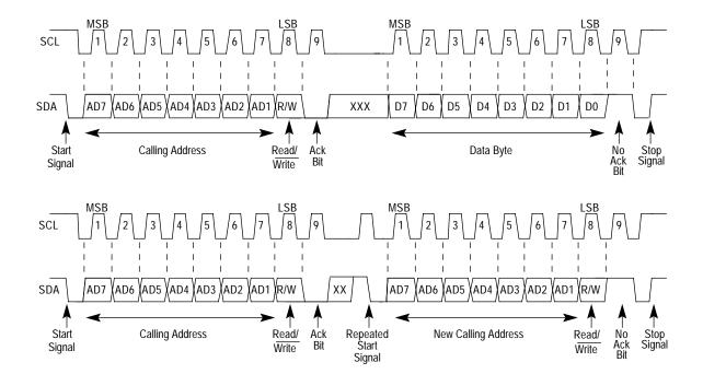
Figure 39 IIC Transmission Signals
