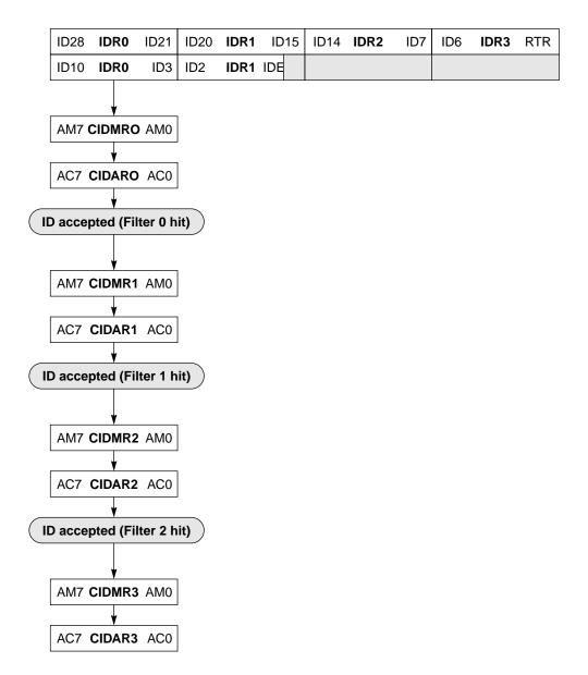
Figure 47 8-bit Maskable Acceptance Filters
