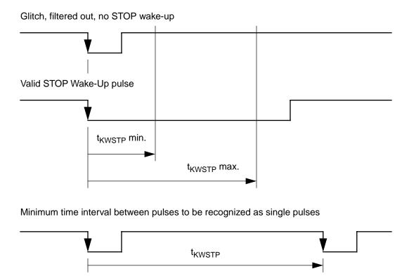
Figure 12 STOP Key Wake-up Filter
