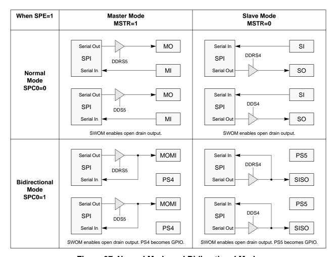
Figure 37 Normal Mode and Bidirectional Mode
