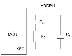
Figure 4 PLL Loop Filter Connections
