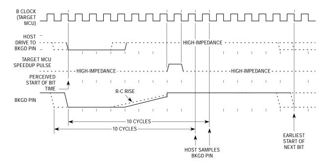
Figure 61 BDM Target to Host Serial Bit Timing (Logic 1)
