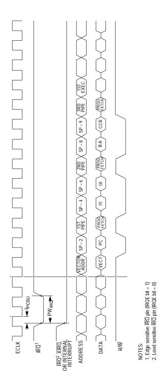
Figure 69 Interrupt Timing Diagram
