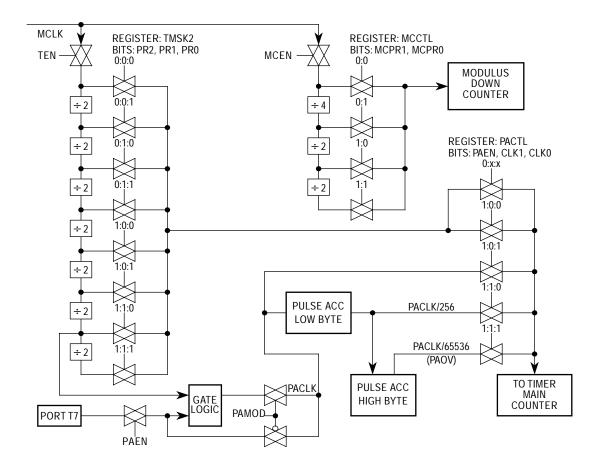
Figure 21 Clock Chain for ECT
