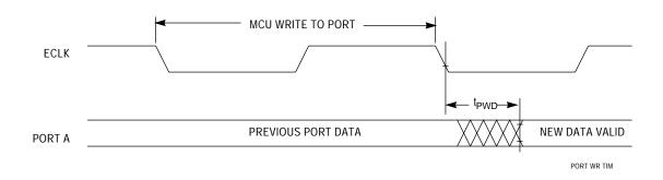
Figure 71 Port Write Timing Diagram
