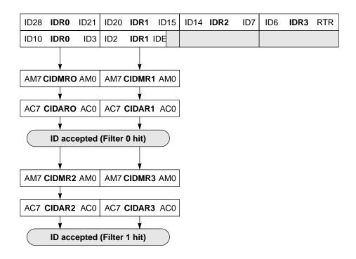
Figure 46 16-bit Maskable Acceptance Filters
