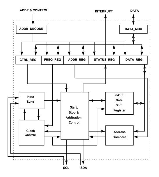
Figure 38 IIC Block Diagram
