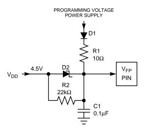
Figure 63 V<sub>FP</sub> Conditioning Circuit
