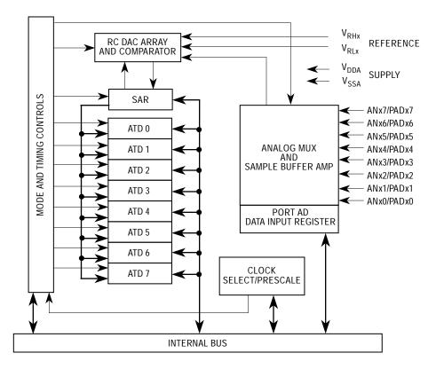
Figure 42 Analog-to-Digital Converter Block Diagram
