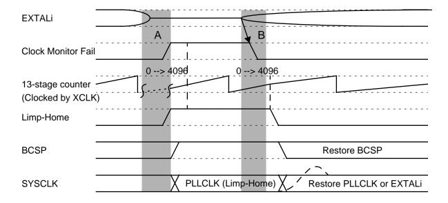
Figure 15 Clock Loss during Normal Operation
