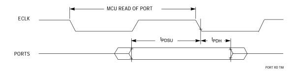
Figure 70 Port Read Timing Diagram
