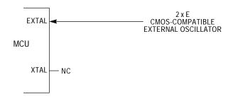
Figure 6 External Oscillator Connections
