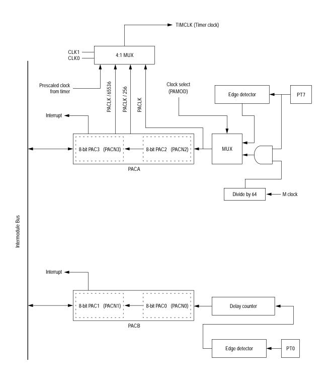
Figure 29 16-Bit Pulse Accumulators Block Diagram
