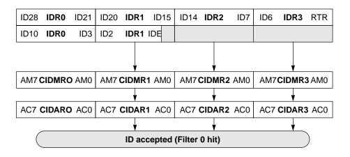
Figure 45 32-bit Maskable Identifier Acceptance Filters
